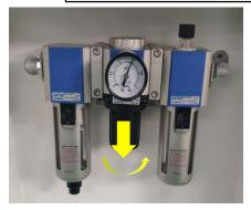
Figure 6-The air supply of the equipment shall not be less than 0.6MP
