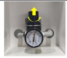
Figure 7- Feeder Pressure 0.55MP
