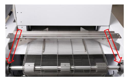
◆Regularly add high temperature lubricating oil to transfer chain bearings.
