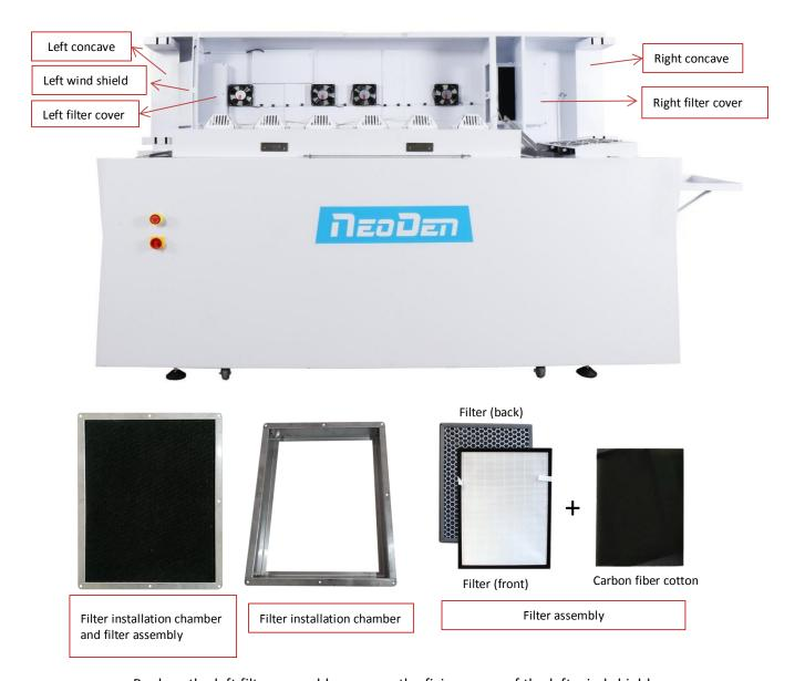
Replace the left filter assembly: remove the fixing screw of the left wind shield and take down the left wind shield --> remove the screw of the left concave and take down the left concave --> remove the fixing screw of the left filter cover and push out the left filter cover to the right --> push out the filter installation chamber and the filter assembly to the right together --> replace the prepared filter assembly and install it in the reverse order of disassembly
