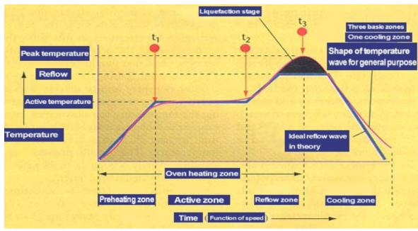
(Fig. 2. Theoretically, the ideal reflow wave consists of four zones, the first three zones are heated and the last zone is cooled.)
