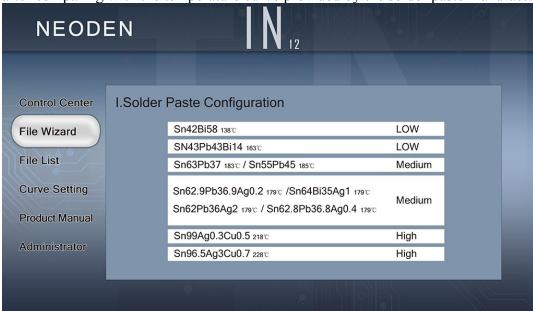
Step 1: select the type of solder paste to solder the product. If the model is not found in the list, please go to search in the appendix, or ask the solder paste manufacturer about the melting point, and then select the option with the closest melting point.
