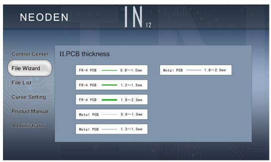
Step 2: select the material and thickness of PCB to be soldered.
