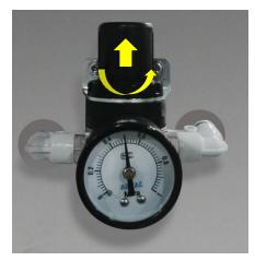
Figure 6-The air supply of the equipment shall not be less than 0.55MP
