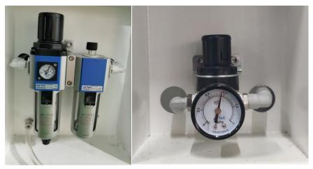
figure 6- oil-water separator
